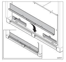
■ Insert the cover for the charcoal filter slots as shown and close it. It is held in place by magnets.
